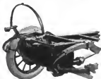
The three-quarter elliptic springs, cylindrical gas tank and tire carrier of the Jeffery
